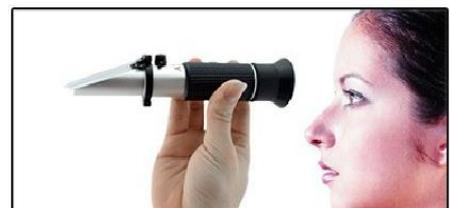
3. Remove cap from adjustment screw, adjust by the use of screw driver, **very gently**, the line between blue (top) and white (bottom) until the line is equal to calibration liquid value.
