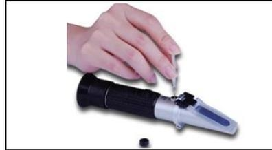
4. Replace protective cap on adjustment screw.
