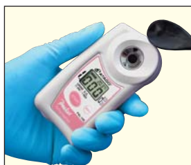
1. Place the sample onto the prism surface.
